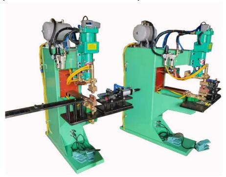
Host, Taiwan water circulation temperature control transformer, Heitian AS2410 large flow electromagnetic, Taiwan electric control box.
